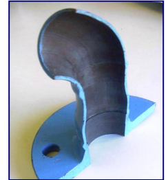
The deposition has been removed and a phosphate layer has been applied
