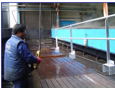
Spray pickling and high-pressure rinsing of aluminium handrails
