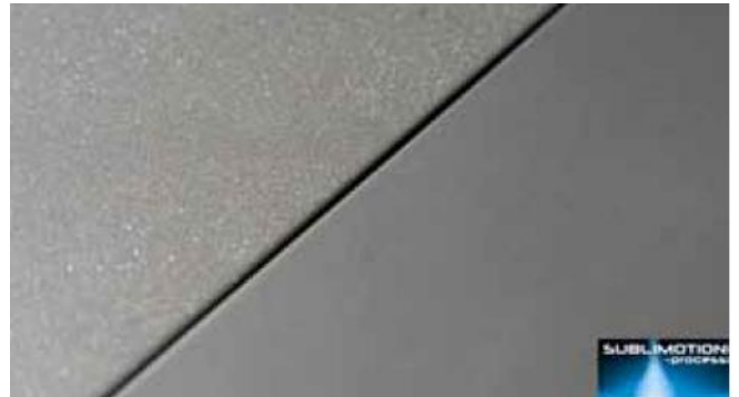
Right: test sheet treated with the SUBLIMATION-process® Left: test sheet treated with conventional bead blasting
