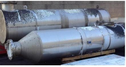
In this acid state, the chloride will severely impair the chromium oxide layer.
