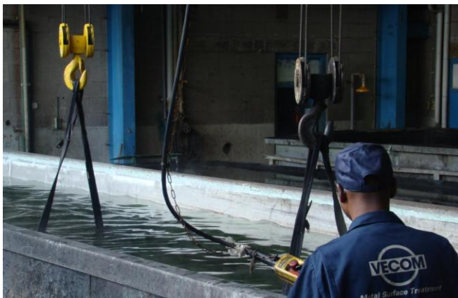
Carbon steel is being immersed in the zinc phosphate bath
