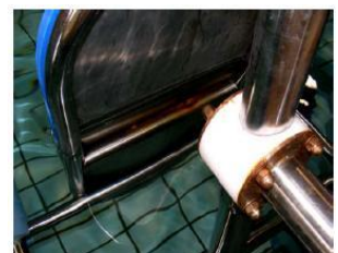
Cleaning with steel wool causes an opposite reaction, namely infection of the stainless steel
