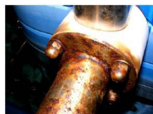
Cleaning with steel wool causes an opposite reaction, namely infection of the stainless steel
