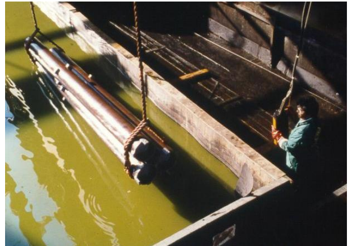
Immersion of carbon steel pipes in a phosphate bath; rust is removed and a phosphate layer remains
