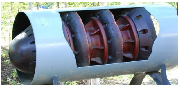
Fig. 1: Pipeline pig demo Trans-Alaska Pipeline (source: www.wikipedia.org)
