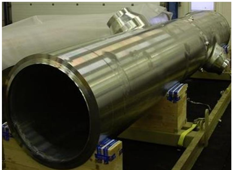
Fig. 3: SS 316 pipe section after pickling treatment. You can clearly see the 91 mm wall thickness on this photo.
