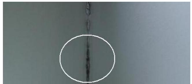
Photograph 2: carbon deposits in a weld seam (here 316L)
