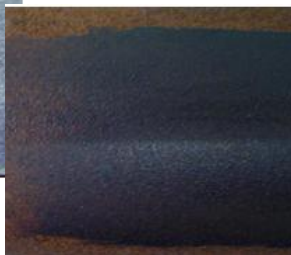
An inert blue/black primer layer has formed
