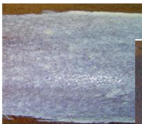
An inert blue/black primer layer has formed
