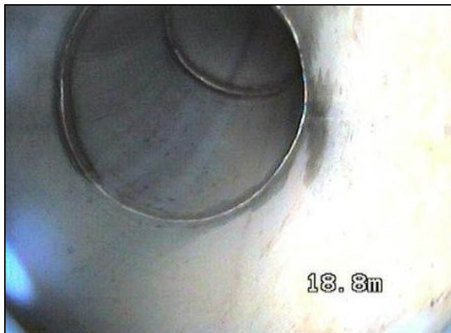
Line 1 – Extensive rust spots, most likely caused by free iron/oxides trapped on surfaces
