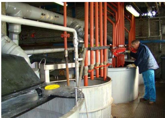
The Vecom mixing drums: various raw materials are mixed to a final product in the drums.
