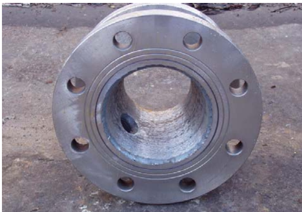
Removal of Japanese Black by mechanical grinding
