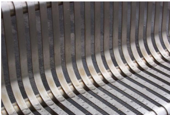
Photo above and below: Corrosion on public stainless steel objects
