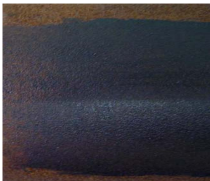
Top: directly after application; Bottom: a blue/black inert layer has formed
