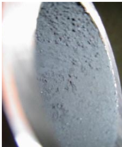
Magnetite layer before cleaning Top right: removed magnetite deposit
