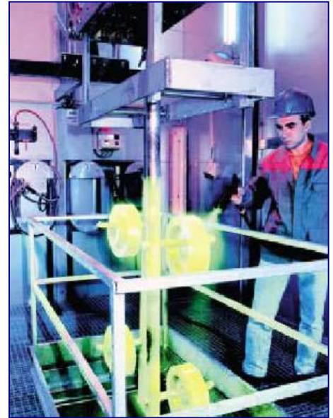
Fluorescent penetrants are faster than the red ones
