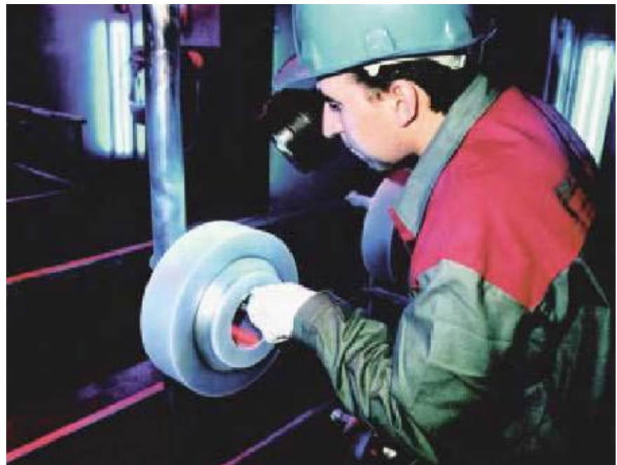
Visual inspection determines the type and seriousness of the defect
