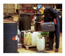
Vecom sampled and coded all the chemicals that were present. The samples – 150 in all – were all analysed in the laboratory so they could be classified. This analysis was important for two reasons: firstly, to establish the chemical composition (based on the general inventory) and, secondly, to determine the best method of processing and recycling and the required fee for this.
