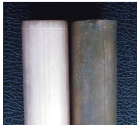
Pickled (left) and not pickled (right) Cunifer tube
