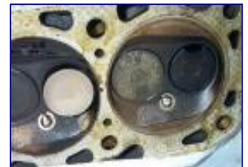
Valve before and after cleaning
