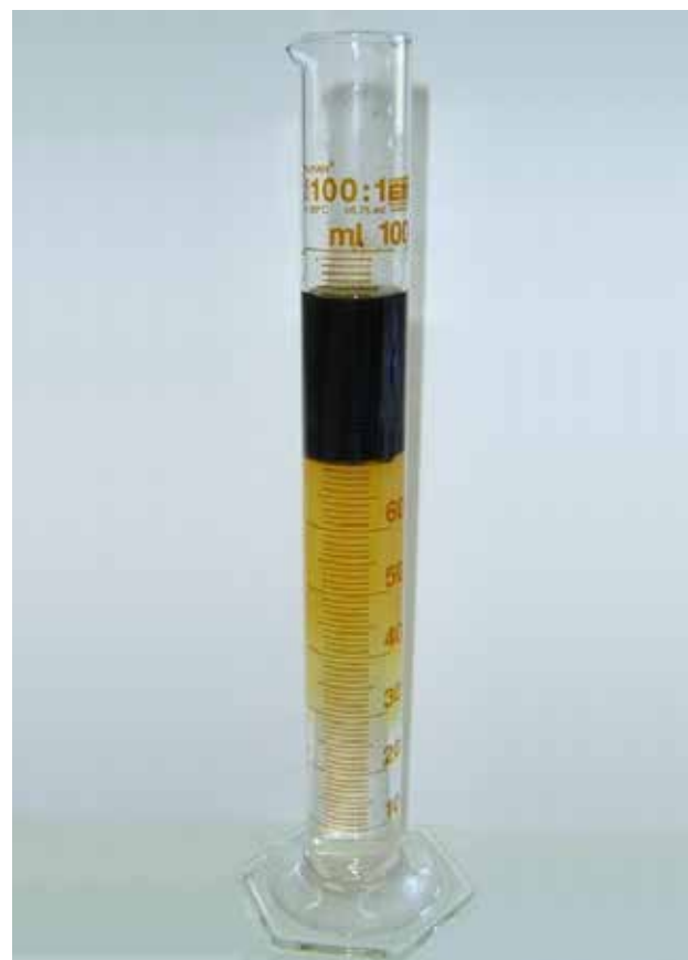
Separation of Veclean LowCOD into an oil and water phase
